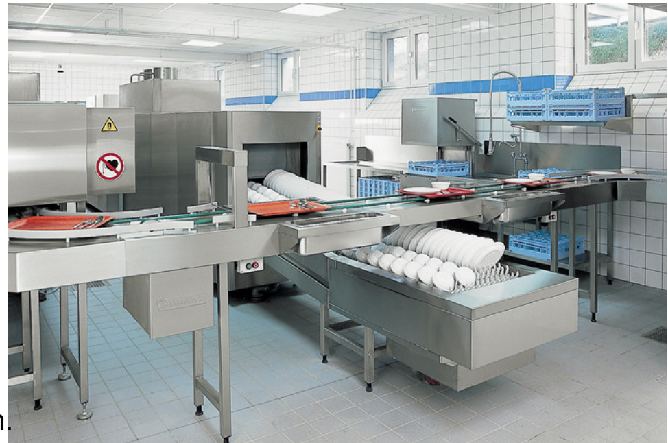
Machine with Lowered Input
