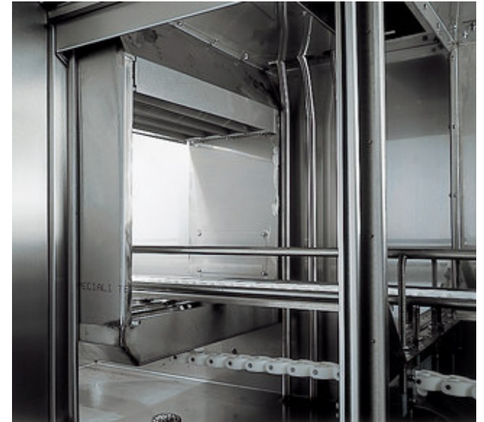
Drying Section With Additional Air Blades
