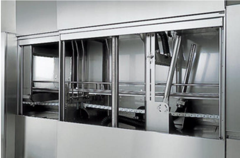
Blowing-Out Zone With Adjustable Air Knives
