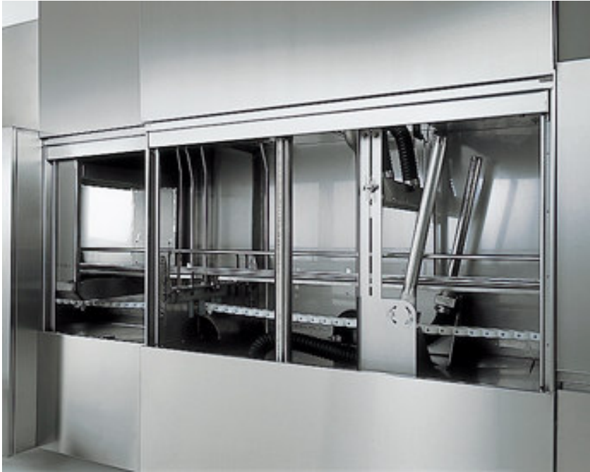
Blowing-Out Zone With Adjustable Air Knives
