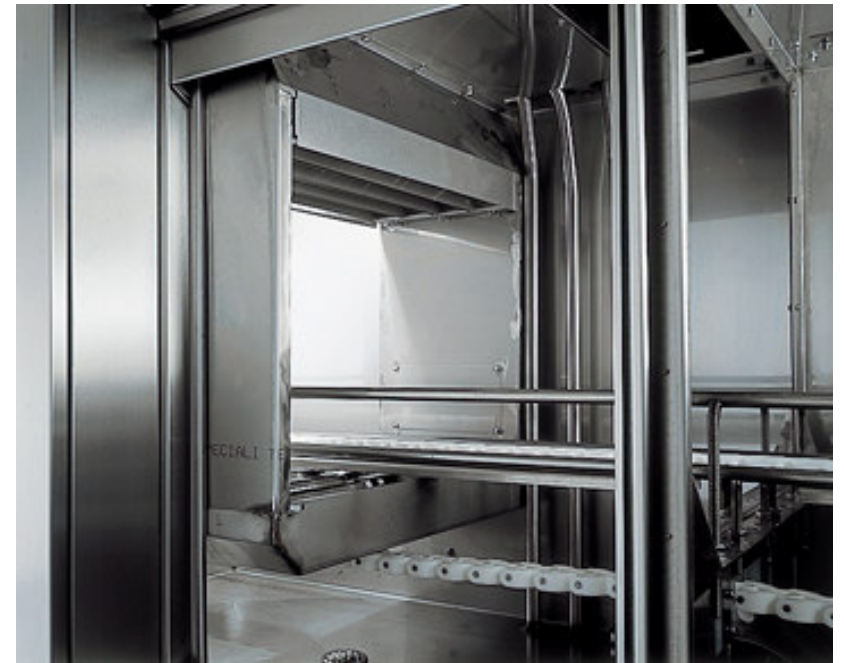
Drying Zone With Additional Air Blades
